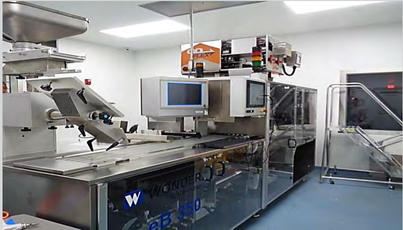
View of Uhlmann eb-350 Blister Pack Machine
