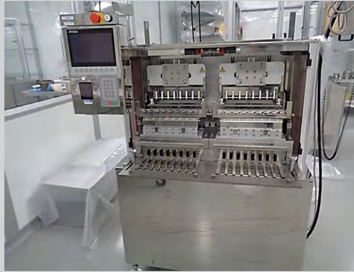
View of Anritsu Capsule Checkweigher
