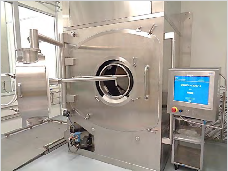
View of Thomas 48" Flex 200 Interchangeable Coating Pan
