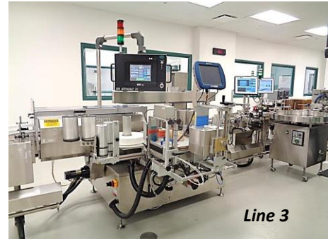
(1 of 3) Cremer 24 & 12 Lane Solid Dose Packaging Lines. Fully automated, late vintage, still installed and operational.
